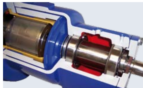
Coated ceramic ZrO 2 shells
