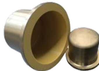
Coated ceramic ZrO 2 shells
